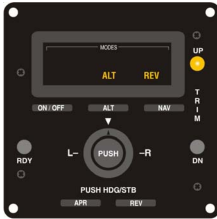
Fig. 2-23. AP Display, REV and ALT HOLD Modes Engaged, TRIM UP Required (System Fifty)
