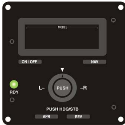
Fig. 2-3. AP Display, RDY for Operation (System Forty)
