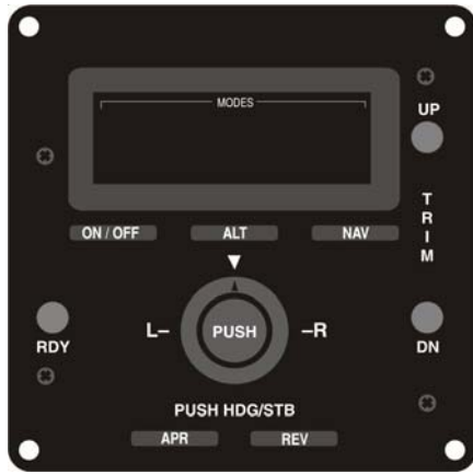
Fig. 2-14. AP Display, All Annunciations and Lamps Extinguished (System Fifty)
